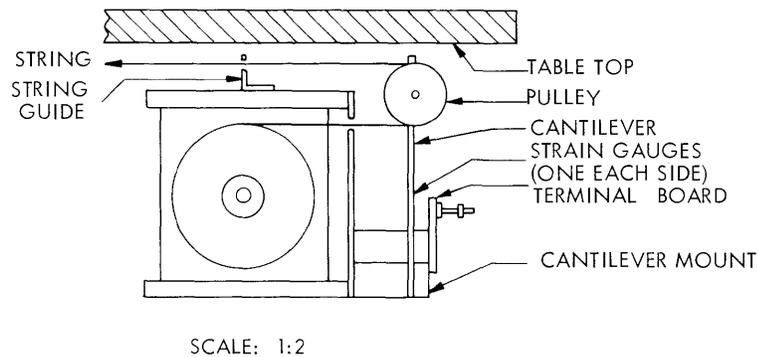
Fig. XIX-11. Cantilever assembly (cross section).
