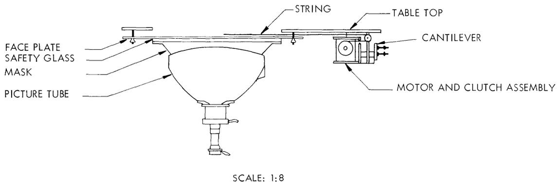
Fig. XIX-12. Picture-tube mounting and transducer.
