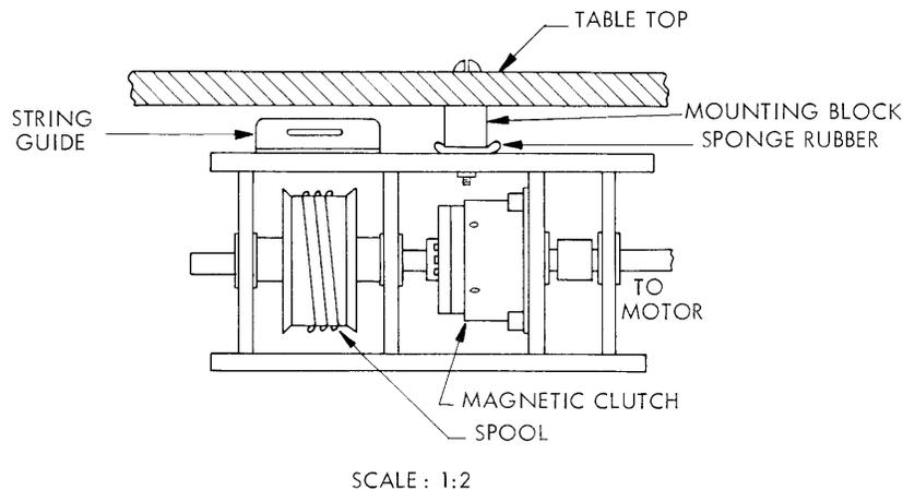
Fig. XIX-10. Clutch assembly (cantilever removed).
