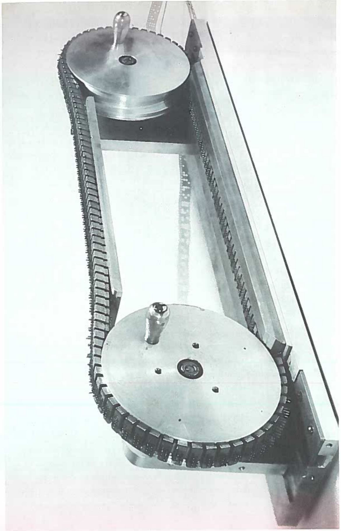
Fig. 4. The pin-type "Braille-out" with wire cable support and spacers between Braille cell blocks.
