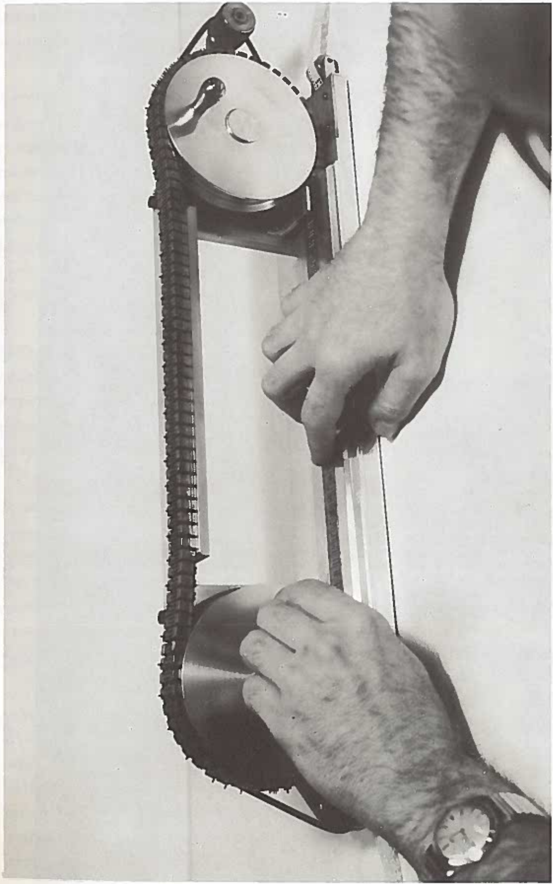
Fig. 1. Punched paper tape to Braille Transducer using a continuous belt carrying pin elements. Device is shown in reading position.
