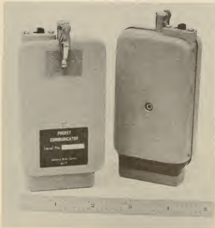
Figure 8 TAC-COM Receivers Front and Rear View.
