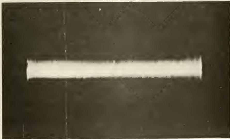
Figure 12. Oscillogram for emission of sine waves of 50 cps under the conditions of Figure 9.
