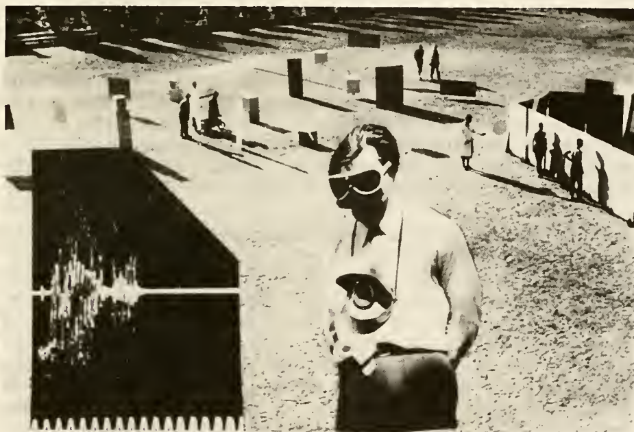
Figure 20. Use of the sonic guiding device worn by a subject (center). The oscillogram at the left shows a single sound impulse with a basic frequency of 400 cps. The obstacle training course used in the tests is shown in the background.
