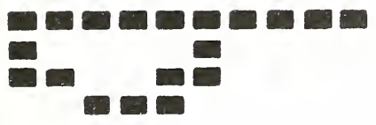
Figure 7. First Stage of Feature Analysis Program: An Examination of the First Column of Digits and Identification, by Comparison with a Mask, of Ascenders, Ribbon Height Verticals, and Descenders.
