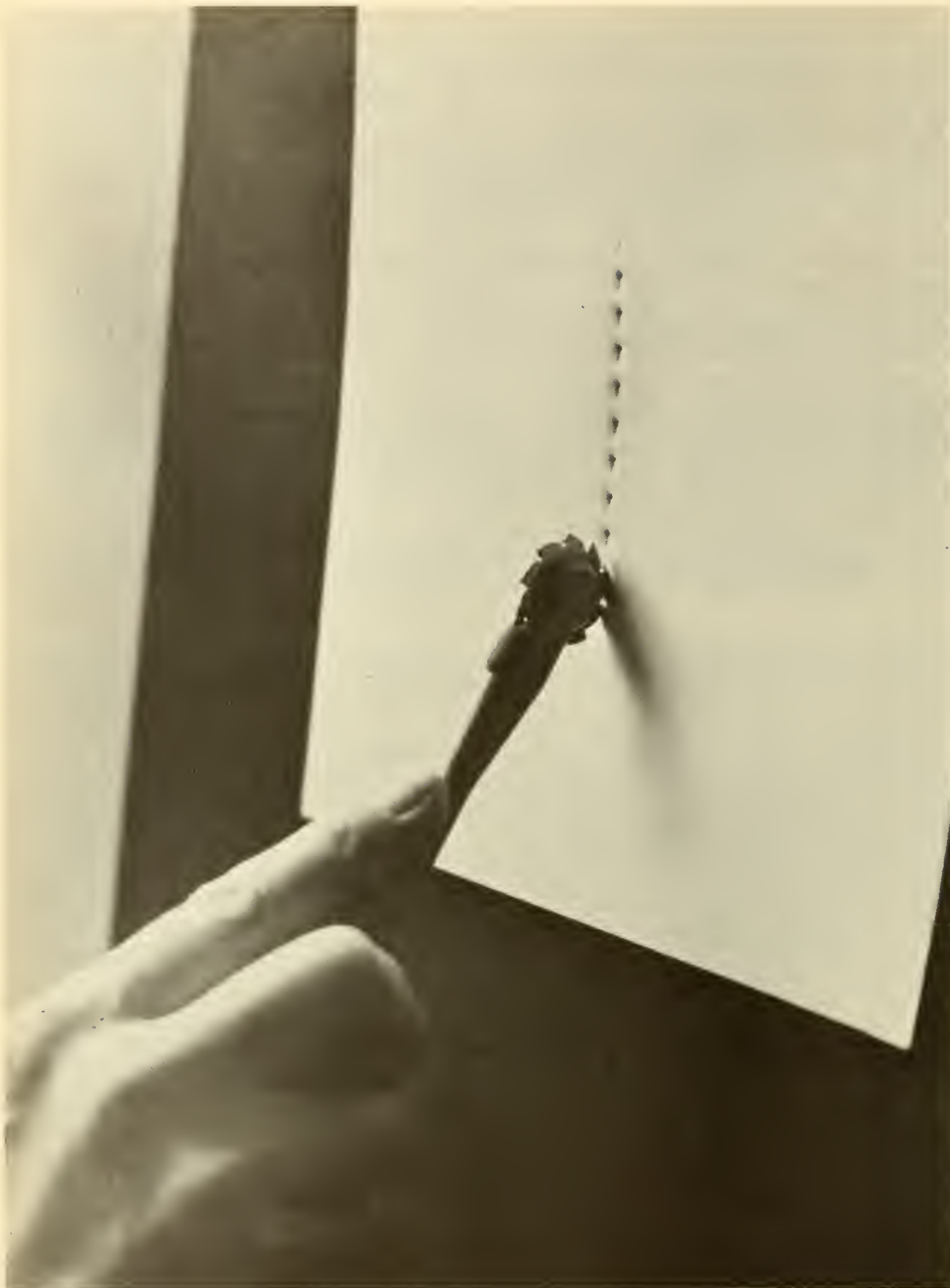
Figure 1. Tactile Symbol Tool Being Used to Make an Impression on an Aluminum Sheet.
