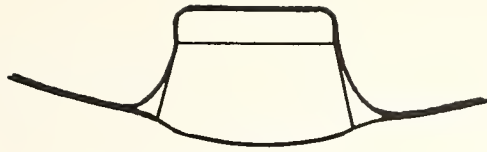
Improper pad shade
