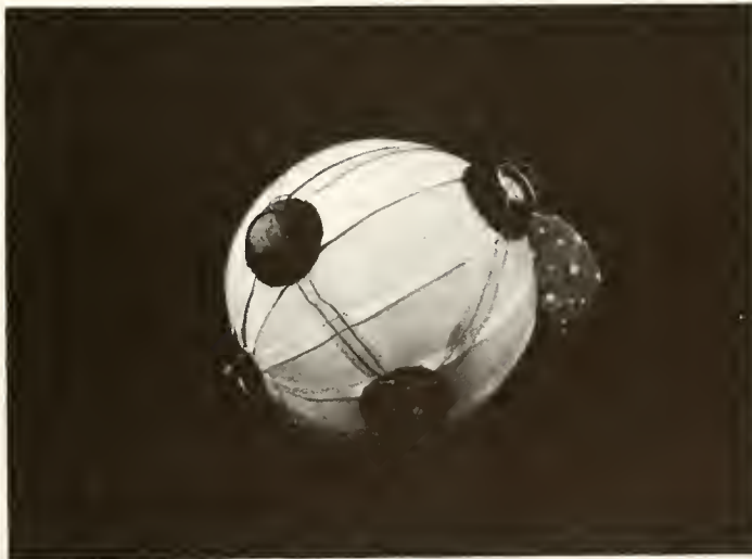
Figure 14. Distributed Component Shell Supported Ball Inside-Out During Construction
