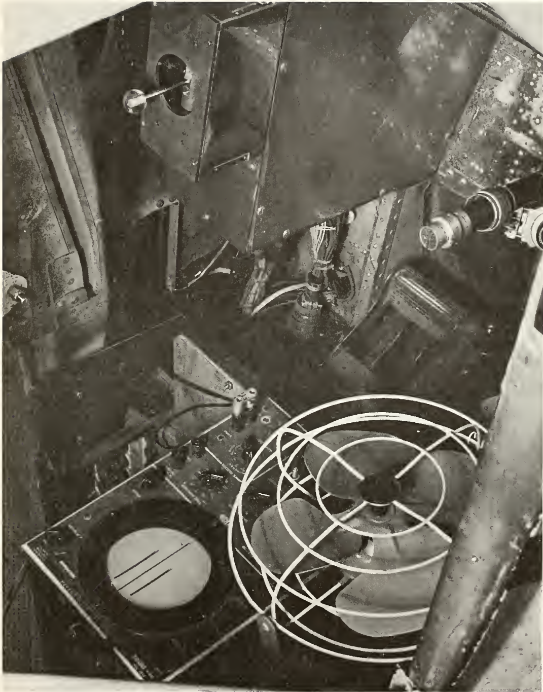
Figure A.2. The Display Scope and the Control Stick Used with the NE-2 Motion Simulator
