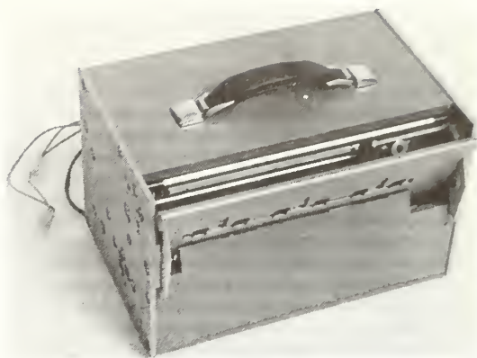
Figure 8. Front Top View of Page Reader, with Spring Door Open, 12 1/2 inches in length.
