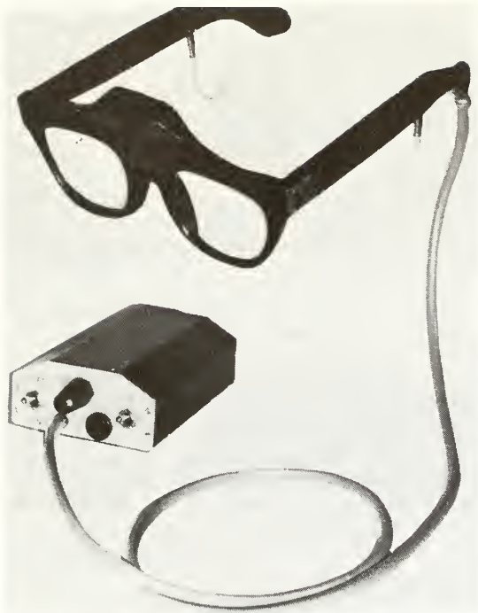
Figure 1. Ultrasonic Binaural Sensory Aid for the Blind
