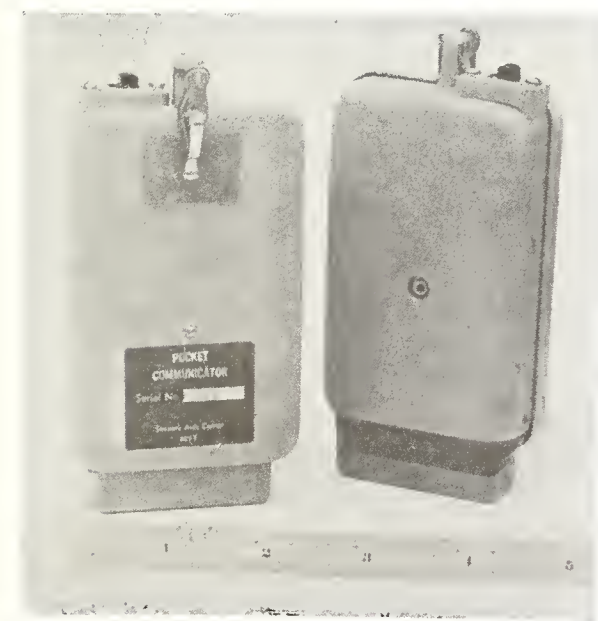
Figure 8. TAC-COM Receivers, Front and Rear View.
