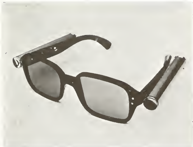
Figure 5. Disassembled view of the prototype eyeglass-mounted infrared mobility aid; transmitter left, and receiver right.
