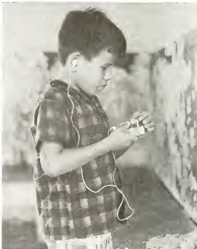
Figure 1. Miniature hand-held infrared mobility aid; a nonranging aid weighing 100 grams, limited to the role of obstacle avoidance when used with a cane or guide dog.
