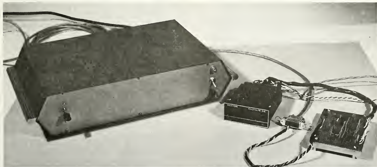
Figure 2. Complete System Including the Numeric Braille Display, Multiplexer Encoder, and Digital Panel Meter.
