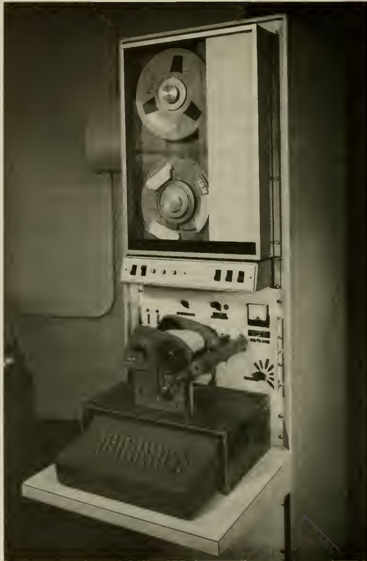
Fig. 2. Monotype Reader, Editing Keyboard and Incremental Magnetic Tape Recorder.
