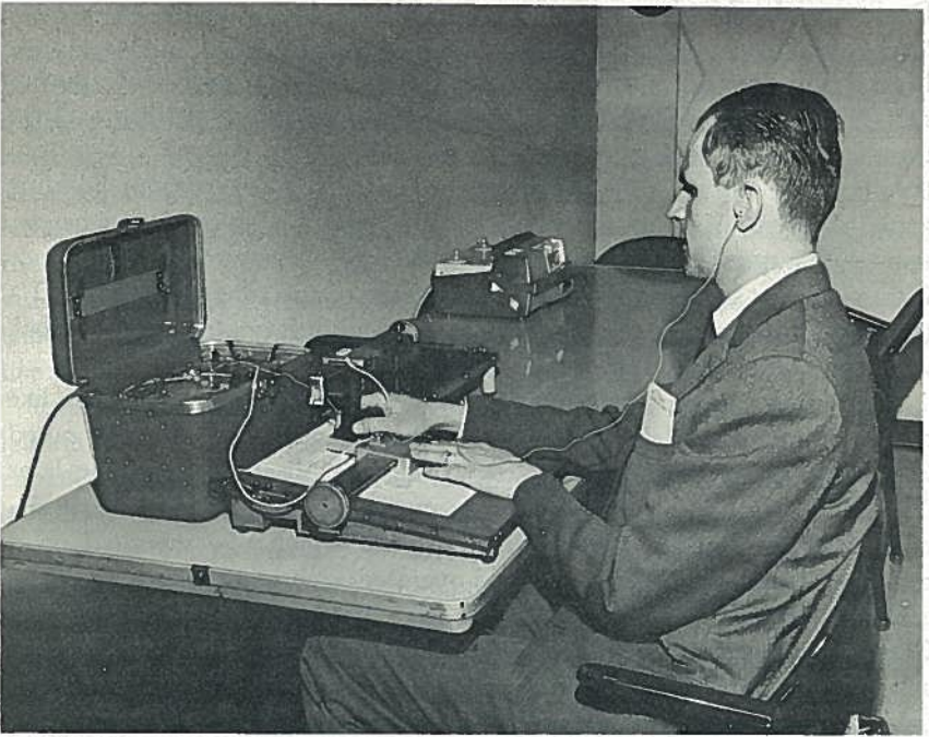
FIGURE 2. Using the VA-Battelle optophone reading aid for the blind. Photocells in the probe which is in the user's right hand convert images of the print on the page to electrical signals which control tones fed through the earpiece. The probe is being guided along the line of print with the aid of a manual tracking device.
