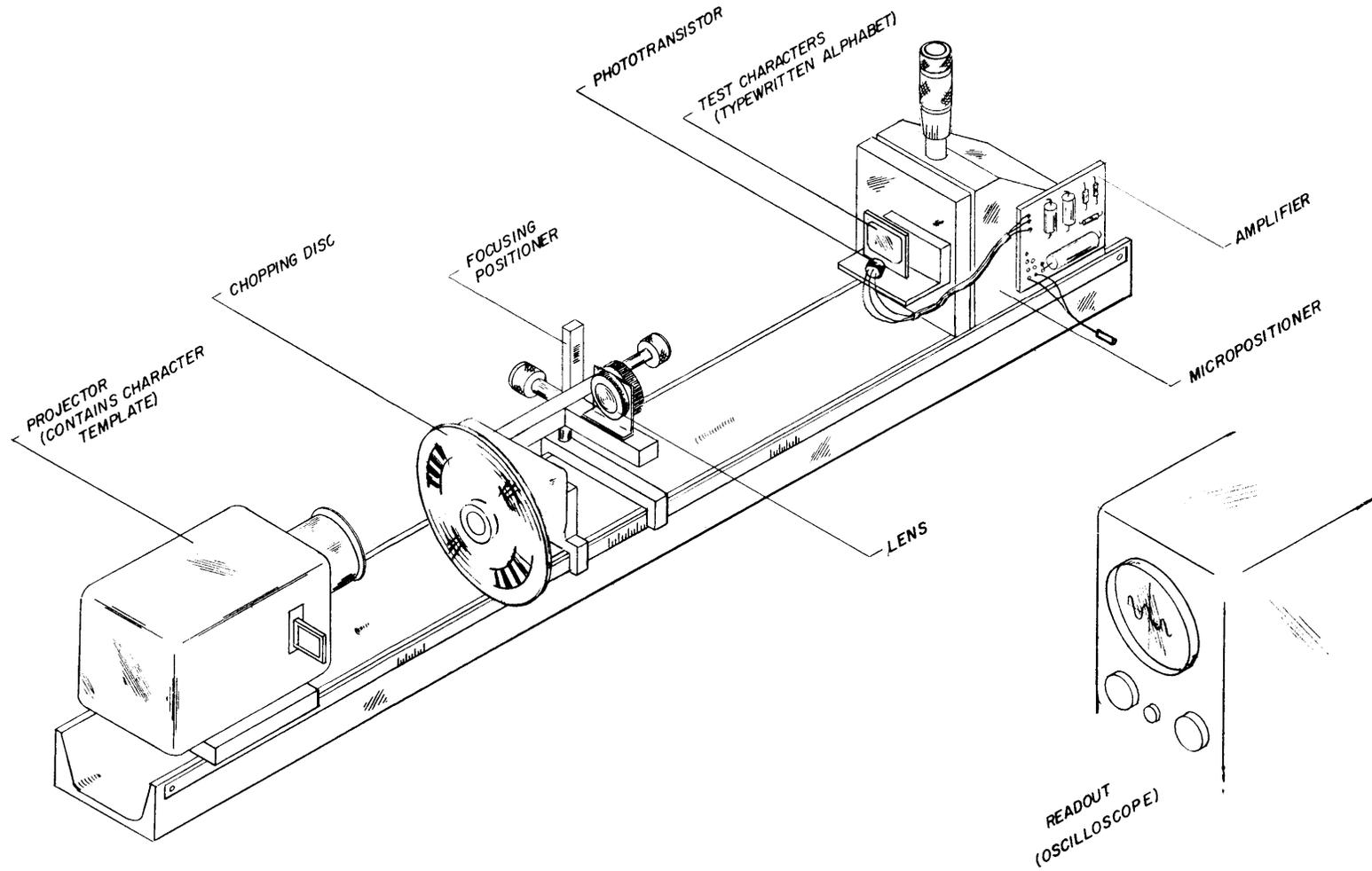
Fig. XIX-4. Optical bench experimental arrangement for evaluation of projected template character comparison technique.
