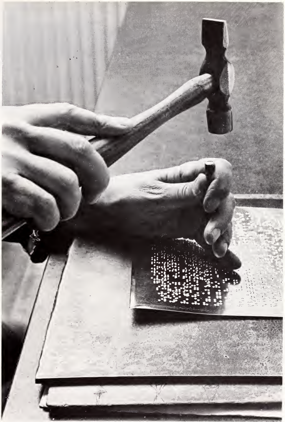
Correcting an error in a braille stereotype plate
